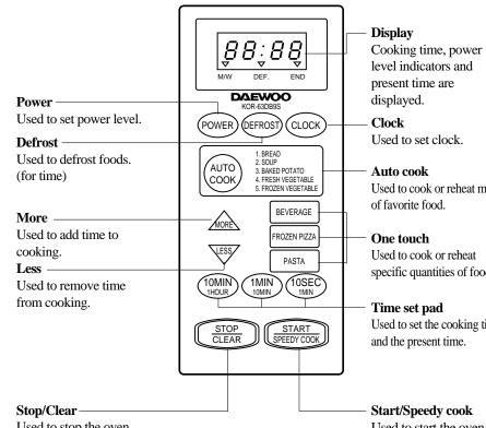
Used to stop the oven operation or to delete the cooking data.
